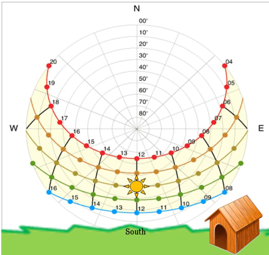
These diagrams can be used to estimate shading for a particular location throughout the year.
