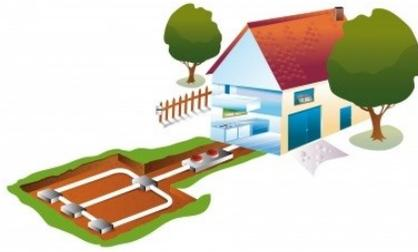
Geoexchange works on the principle that within a few feet of the surface, the earth remains a nearly constant temperature year round. In winter the ground is slightly warmer, and in summer slightly cooler than the air. Geoexchange simply moves and compresses the low grade temperature difference (heat or
