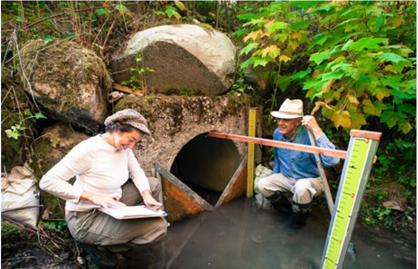
Weir at Yasodhara Ashram measures flow. This weir is available for relocation.
